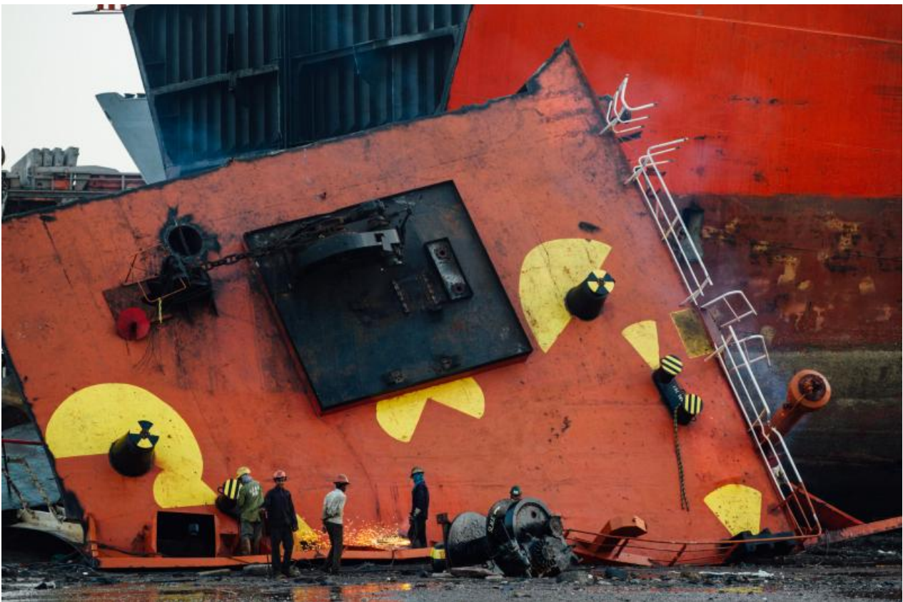
Acetylene Cutting Torch, Shipbreaking at Alang Shipyards in India. Photo: Adam Cohn. View source .
